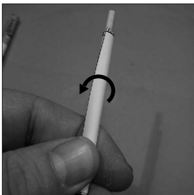
Roll C around a thin dowel. The gluetabs shall be on the outside.
